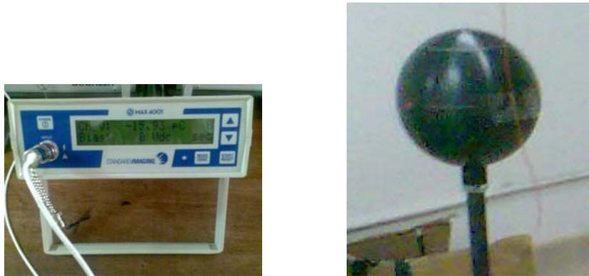
**Gambar 1.** Elektrometer Standard Imaging model MAX-4001 no. seri N063072 dan detektor Exradin model A6 no.seri XQ063051
