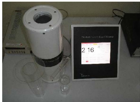
Gambar 1. Alat ukur Dose Calibrator Mark VI
