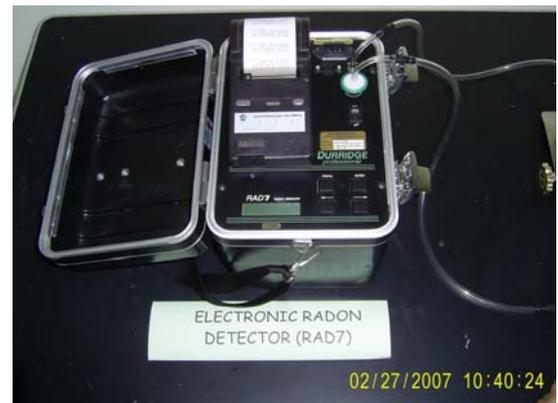
Gambar 1. Alat *electronic radon detector RAD 7*
