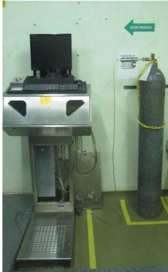
Gambar 2. Alat Hand and Foot Monitor
