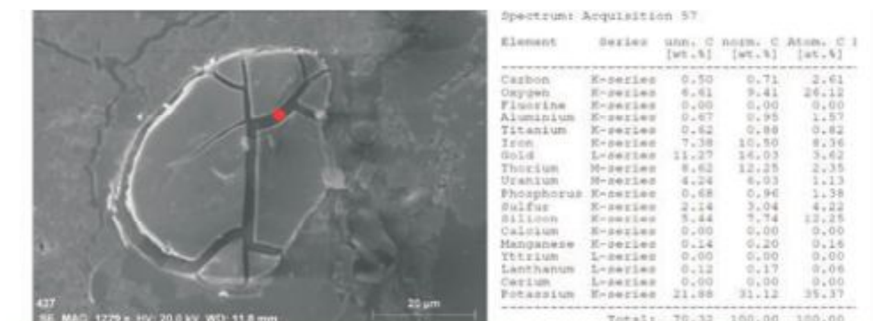
Figure 10 Point analysis in fracture of thorianite minerals showing the uranium content higher than in the minerals body
