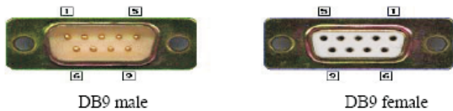
Gambar 2: Pin DB9. Keterangan : Pin 1 = Data Carrier Detect (DCD), Pin 2 = Received Data (RxD), Pin 3 = Transmitted Data (TxD), Pin 4 = Data Terminal Ready (DTR), Pin 5 = Signal Ground (Common), Pin 6 = Data Set Ready (DSR), Pin 7 = Request To Send (RTS), Pin 8 = Clear To Send (CTS), Pin 9 = Ring Indicator (RI)
