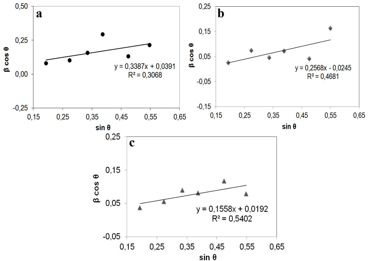
**Figure 2.** Relation curve of ( $\beta \cos \theta$  versus  $\sin \theta$ ) on composite of  $Ba_{(1.5)}Sr_{(0.5)}Fe_2O_5$  with various sintering temperature (a)  $T_1 = 800 \text{ }^\circ\text{C}$ , (b)  $T_2 = 900 \text{ }^\circ\text{C}$ , and (c)  $T_3 = 1000 \text{ }^\circ\text{C}$ .
