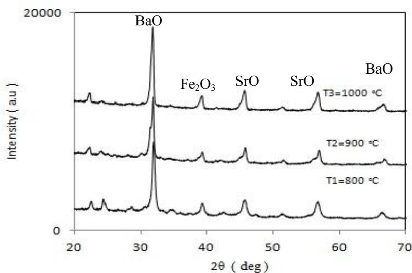
**Figure 1.** Phases identification of  $Ba_{1.5}Sr_{0.5}Fe_2O_5$  X-ray diffraction peak.
