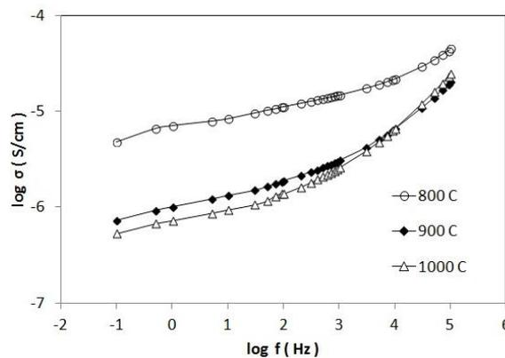
**Figure 3.** Conductivity value of  $Ba_{1.5}Sr_{0.5}Fe_2O_5$ .
