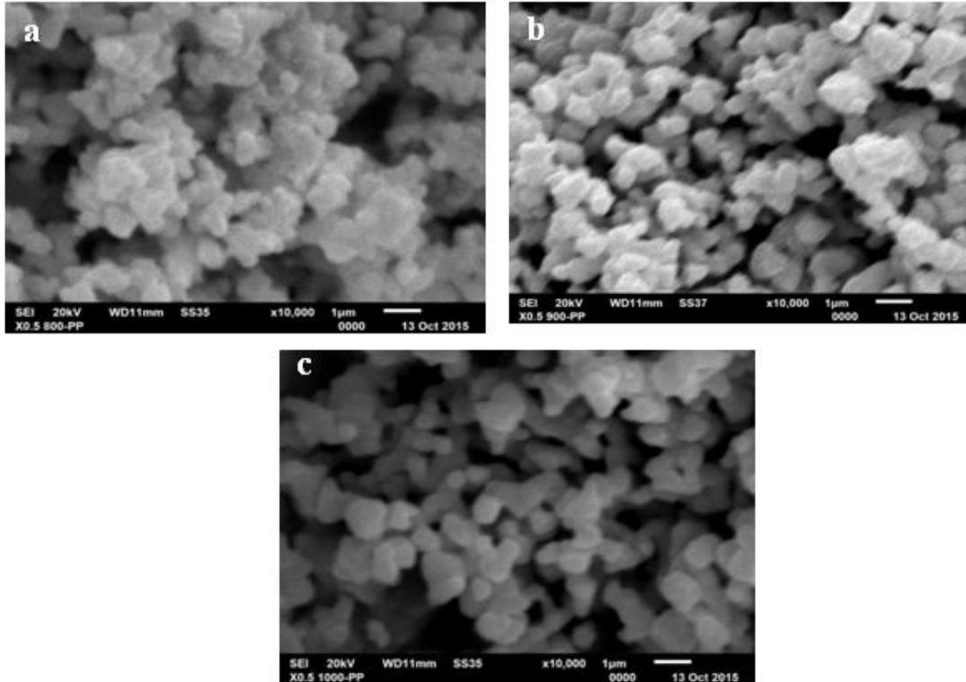
**Figure 4.** Surface of  $Ba_{1.5}Sr_{0.5}Fe_2O_5$  and Spectrum EDS with various sintering temperatures (a)  $T_1 = 800 \text{ °C}$ , (b)  $T_2 = 900 \text{ °C}$ , and (c)  $T_3 = 1000 \text{ °C}$ .
