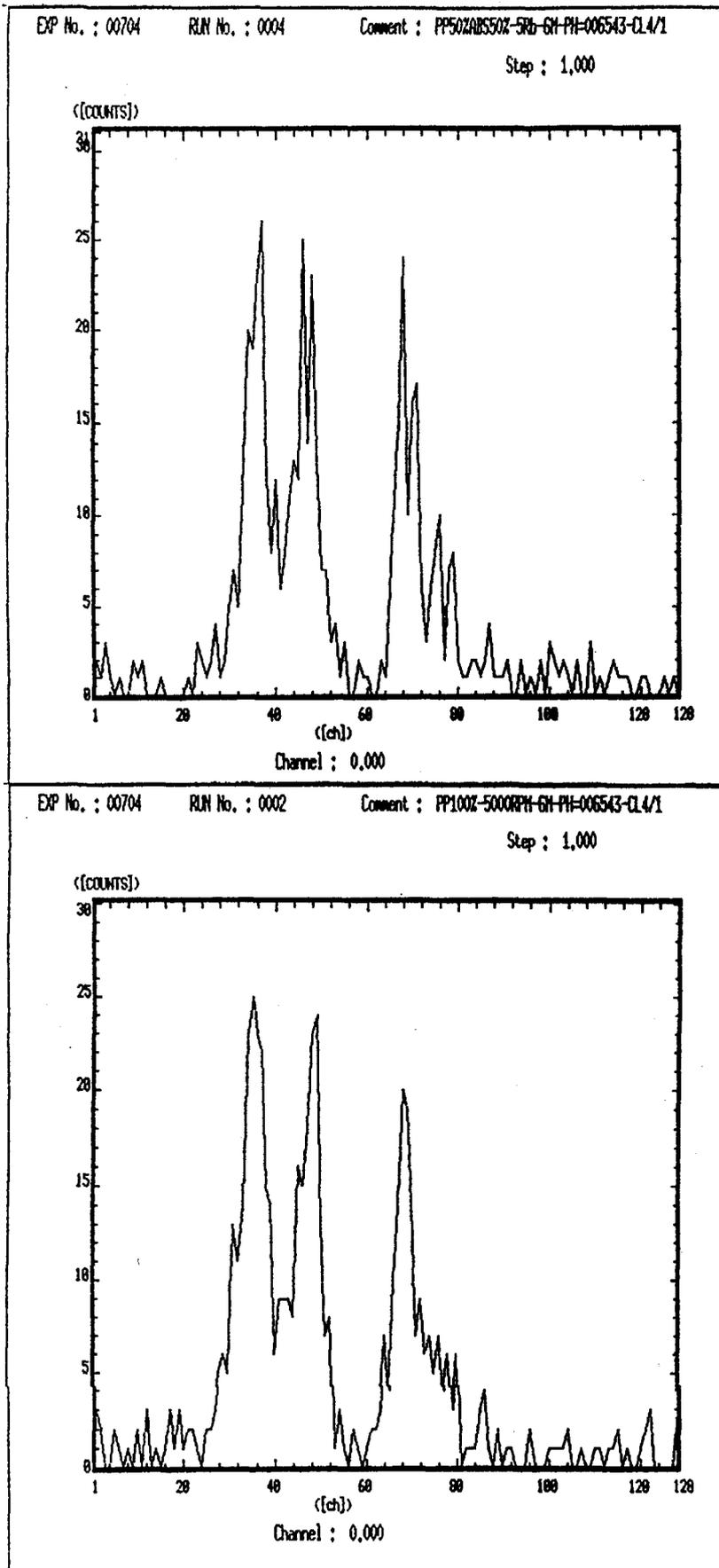
**Figure 6** SANS profiles of 50% ABS - 50% PP (TOP) and 100% PP (BOTTOM)
