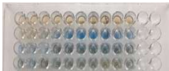
Figure 4: Colorimetric test of DOTA-PAMAM G3 fractionation purification result with Coomassie Brilliant Blue G-250 dye protein
