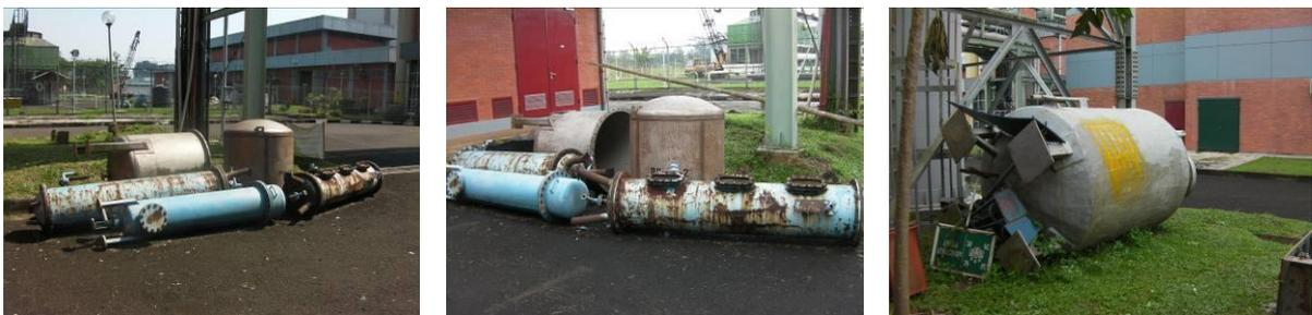
Gambar 11. Keadaan kondisi terkini alat *demineralized water*
