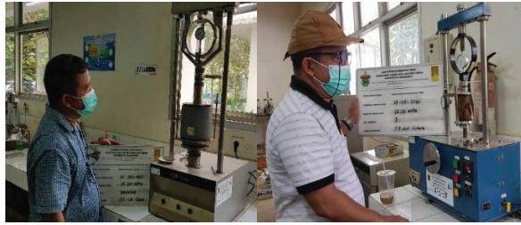
Gbr. 3. Pengujian CBR Test dan Unconfined Compression Strength Test.
