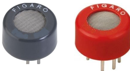
Gambar 1. Jenis sensor gas hidrogen SnO 2 [2]
