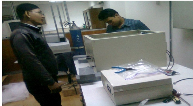
Gambar.1 Instalasi alat Alpha Beta Counter G520
