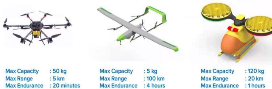
Figure 9. Maximum Capacity, Range and Endurance of Drone type [Source; Terra Drone Indonesia]
