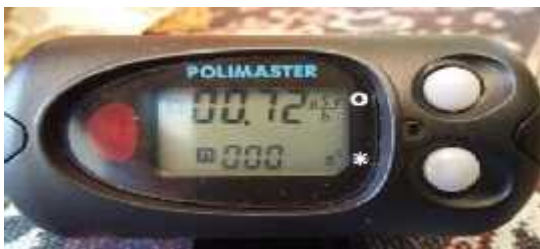
Figure 1. An environmental radiation monitoring instrument showing a dose rate of 0.72 \mu\text{Sv h}^{-1} in area with high natural radiation of Botteng.
