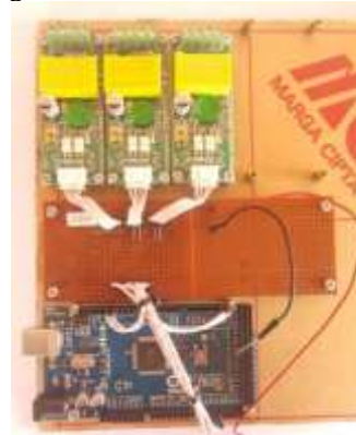
Gambar 2. Hasil Perakitan Sensor PZM004T
