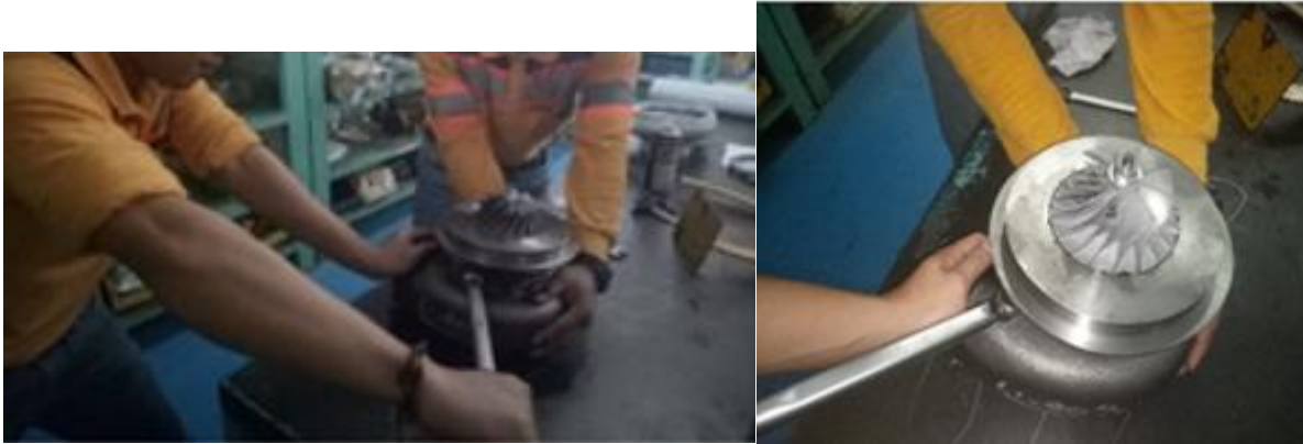
Gambar 3. Proses assembly komponen turbocharger.
