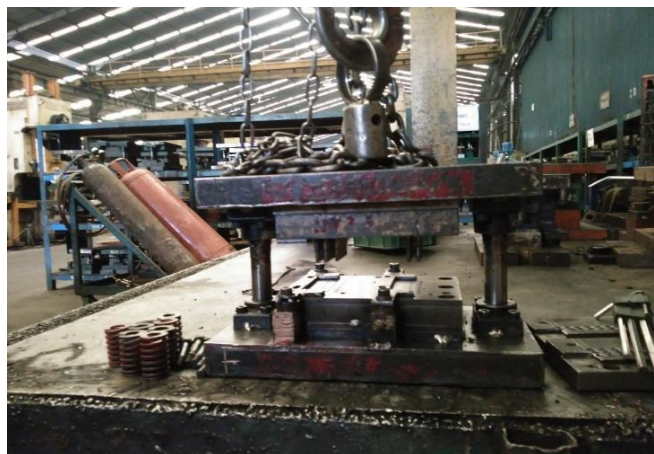
Gambar 5. Proses assembling dies
