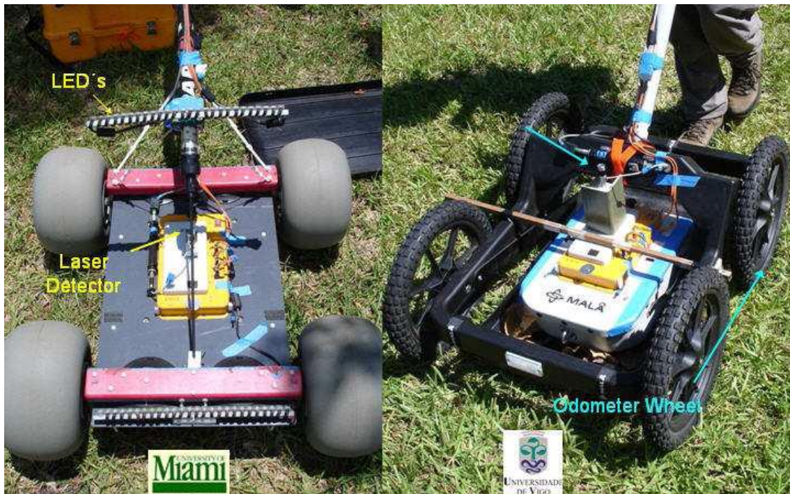
(Foto 1: GPR (Ground Penetrating Radar))
