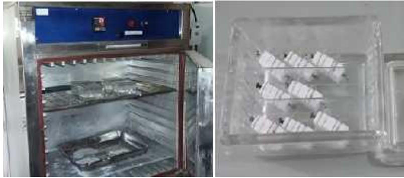
Figure 5. The etching process detectors CR-39 by using 6.25 N NaOH at 70\pm 2 °C in oven for 7 hours.
