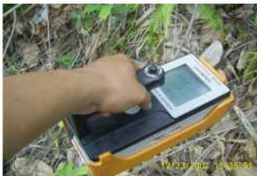
Figure 2. Gamma dose rate measurement by using EXPLORANIUM GR 130
