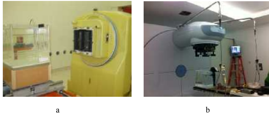
Figure 2. Irradiation set-up using an Alcyon 60 Co machine owned by the Secondary Standard Dosimetry Laboratory of PTKMR-BATAN used as a low activity calibration source (a) and a 60 Co Gamma Beam 100-80 External Beam Therapy System owned by the Dr. Kariadi General Hospital Medical Centre, Semarang used as a high activity source (b)
