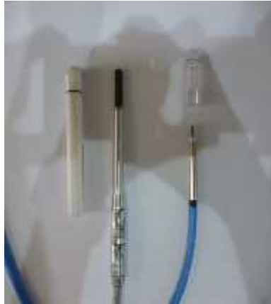
Figure 1. Small volume ionization chamber Pinpoint type PTW 31016 volume 0.016 cc and standard ionization chamber type TW 30013 volume 0.6 cc.
