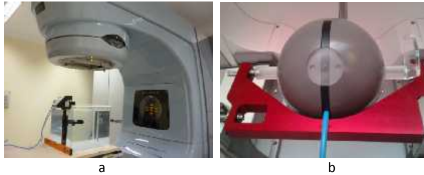
Figure 4. The irradiation set-up of the measurement for the testing of the calibration result of a small volume ionization chamber type PTW 31016 serial number 004507.
