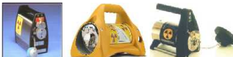
Figure 1. Three types of portable gamma radiography camera are utilized in Indonesia.
