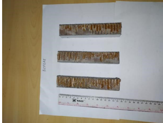
FIGURE 10. Specimen Three-point Bending Vinyl Ester-Sandwich Composite Structure before Test
