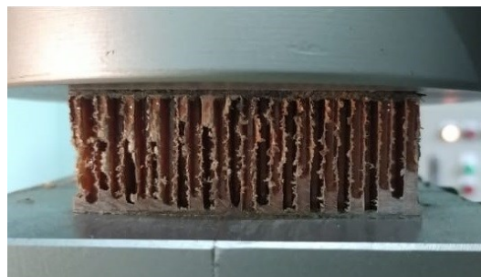
FIGURE 5. Flatwise Compressive Test
