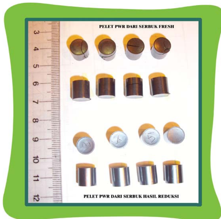
Pelet UO 2 hasil riset / UO 2 pellets of research product
