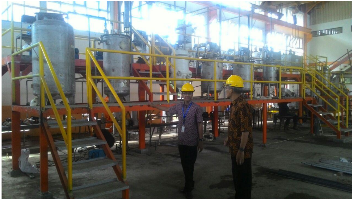
• Gambar 2. PLUTHO Project (Pilot Plant Kapasitas 50 kg monasit/hari)
