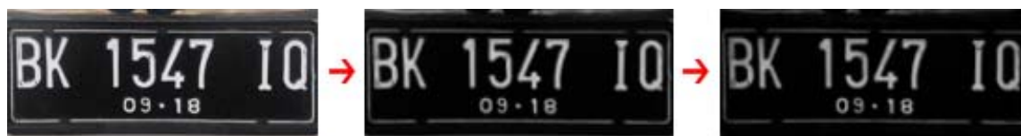
Fig. 1. (left) An example of a valid number plate sample, (middle) gray scaled image and (right) resulted image form top-hat transformation.
