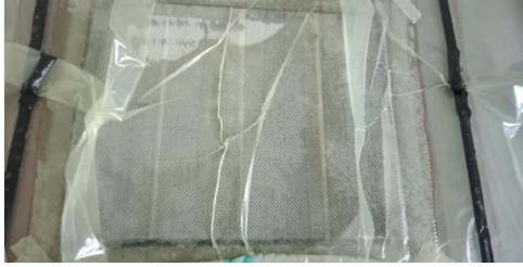
Gambar 2. Proses Vacuum Assisted Resin Infusion (VARI)
