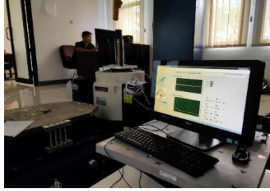
Figure 1. Accelerometer sensor validation activities using a vibration test system
