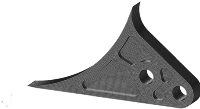
Gambar 4. Model elemen hingga lug fitting
