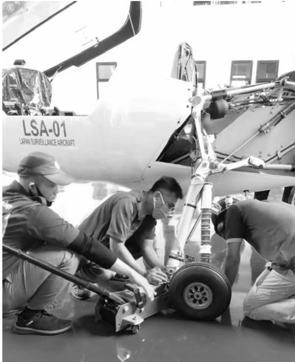
**Gambar 4.** Inspeksi *main landing gear*
