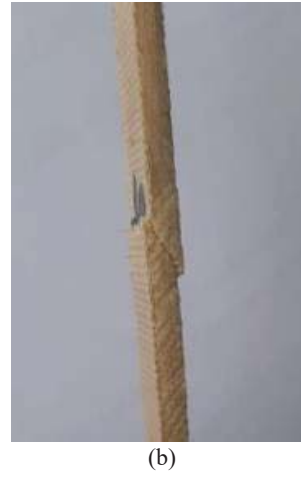
FIGURE 8. (a) compressive strength of e-glass/vinyl ester and (b) compressive failure mode.
