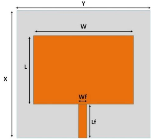
Fig. 2. Rectangular Patch Microstrip Antenna Design
