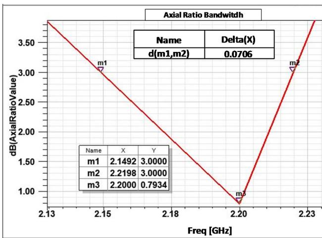
Fig. 8. Bandwidth Axial Ratio of Truncated Corner Antenna
