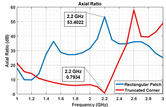
Fig. 7. Axial Ratio of Rectangular Patch & Truncated Corner
