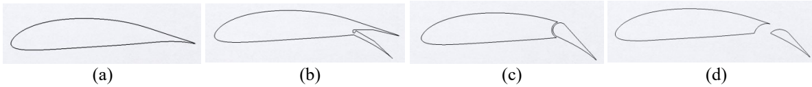
FIGURE 2. 2D Geometry Model of Airfoil FX 76-MP-160: a. No Flap, b. Split Flap, c. Plain Flap, d. Slotted Flap
