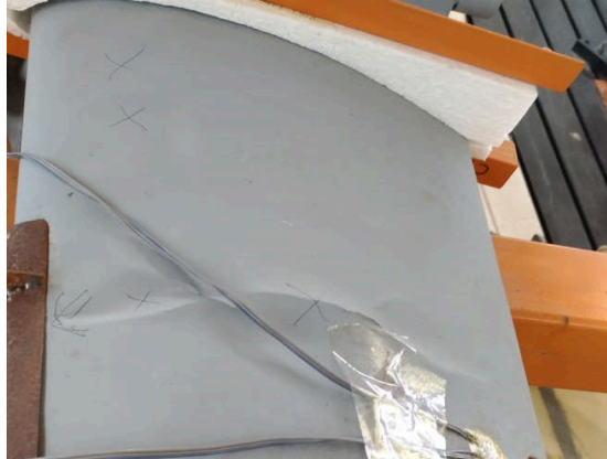
FIGURE 5. Buckling on skin of LSU-02 NGLD's wing.
