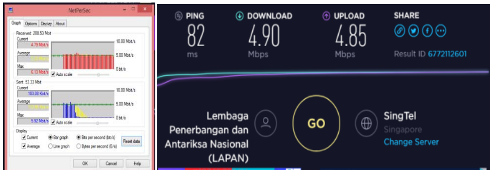
Gambar 3-3: Hasil speed test setelah traffic shapping Eselon IV
