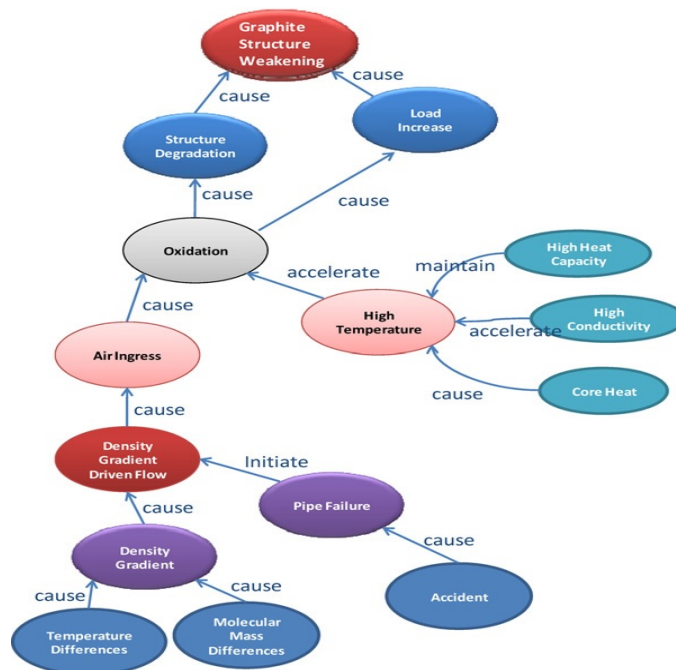
Figure 1. Root causes of air-ingress accident [17,19]
