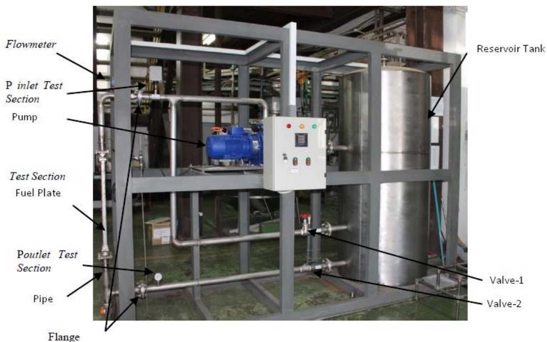
Figure 2. The Channel Experiment Facilities (ExNal) [1]
