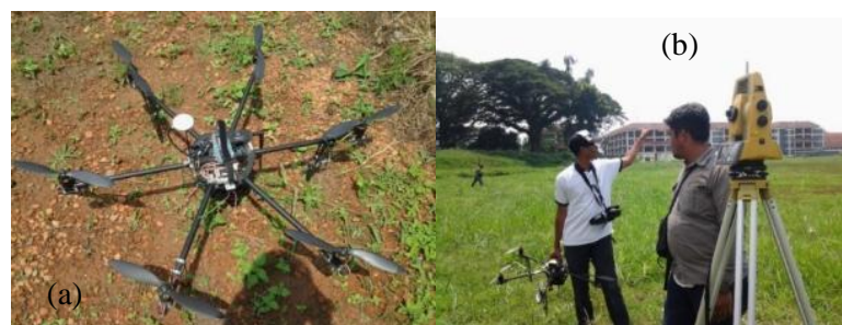
Figure 3. Preparation of HexaCopter (a) and Robotic ETS (b)
