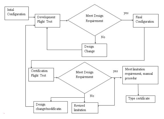
Fig. 2.1. Several step related to flight test activitiy to get type certificate
