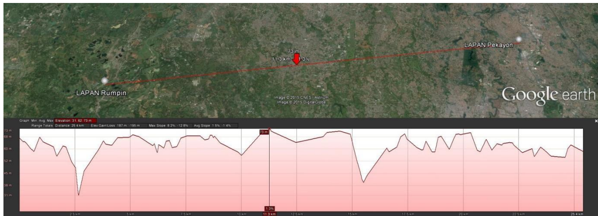
Gambar 3-1 Path Profile Jalur Komunikasi Radio Microwave (Google Earth)
