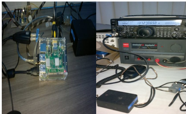
Figure 3-2 Raspberry Pi Connect to Transmitter via Interface
