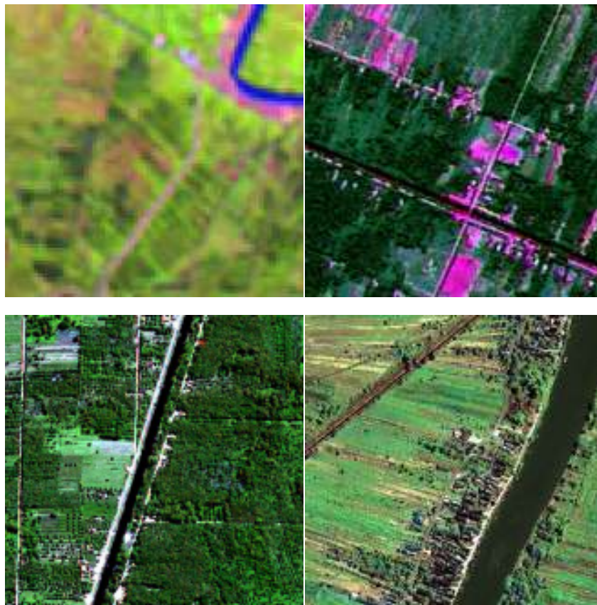
Figure 6.2.1: Landsat and high resolution imagery for a sample area in central Kalimantan. Top left: 2009 Landsat TM image (25m) bands 3,4,5 in BGR. Top right: Pan-sharpened SPOT 5 image (2.5 and 10m). Bottom-left: Pan-sharpened SPOT 6 (1.5m). Bottom-right: Pan-sharpened Quickbird (0.6m and 2m). Individual trees can be seen in the Quickbird and SPOT 6 imagery which is suitable for LCCA purposes. Land cover can be inferred from the SPOT 5 imagery but more interpretation is required.
