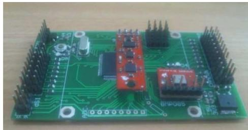
Gambar 3-8. *Flight Controller* Hasil Penelitian Buatan APTRG.
