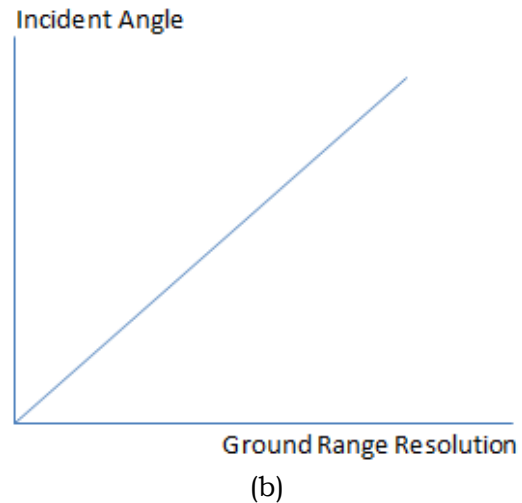
Figure 4-3: Comparison graph of incident angle to: (a) ground swath width, (b) resolution of ground range
