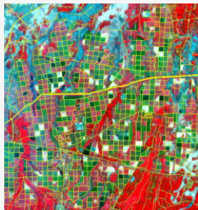
Fig. 19 Results cubic convolution resampling overlay with vector data path and the river RBI 1:25.000
