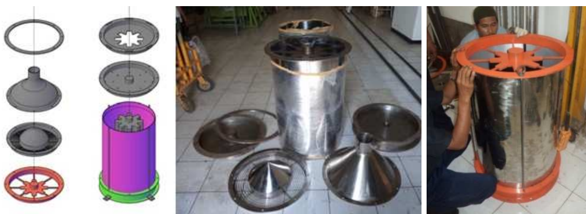
Gambar 3.2 Rancang Bangun Alat Casting D550 Case Bonded
