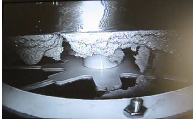
Gambar 4.3 Slurry propelan melewati slitter plate
