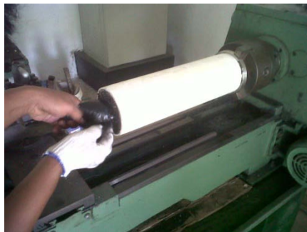
Gambar 2.3a. Loading material liner
