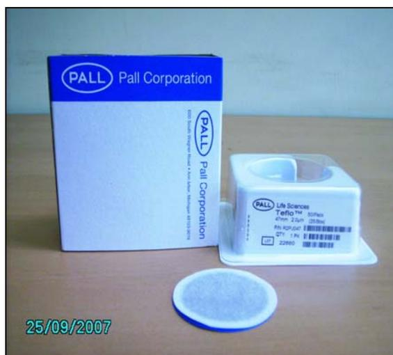
Gambar 5. Filter teflon berdiameter 47 mm.
