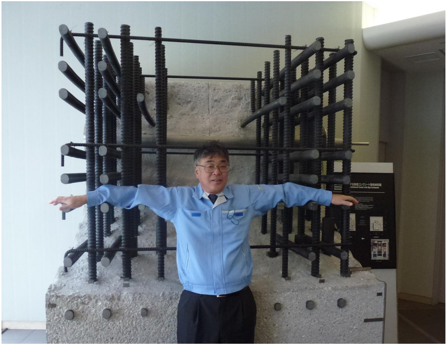
Concrete of containment vessel of BWR(about 2m)
