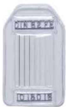
Figure 7. Image Quality Indicator (IQI) DIN 62 FE – 10 ISO 16 which contains 7 wires [14].
