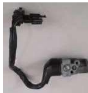
Figure 1. Specimen for fluoroscopic examination is a ignition house of motor bike made of soft-alloy casting material.
