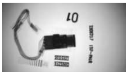
Figure 4. Fluoroscopic image generated from x-ray voltage of 270 kV and current 5 mA.
