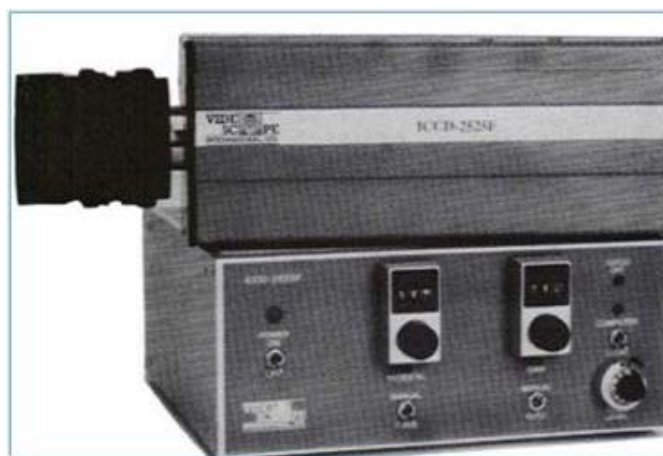
Gambar 3: Kamera ICCD Videoscope.
